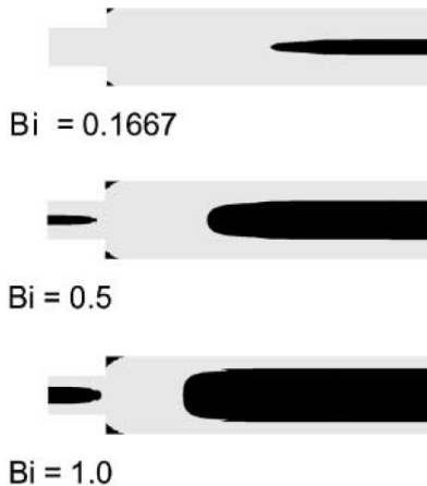
Figure 7: Progressive growth of the unyielded region (shaded) in entry flow through a 2:1 planar expansion of viscoplastic fluids obeying the Herschel-Bulkley-Papanastasiou model with M=1000 , n=0.5 , Re=1 [47]. The flow is from left to right.
